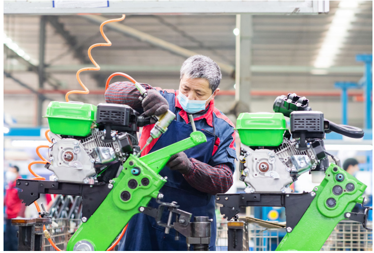
January 17, 2022: A worker assembles a tiller designed for agricultural work in mountainous areas at Chongqing Shineray Agricultural Machinery Co., Ltd. In 2021, the company's products were exported to more than 80 countries and regions including India, Russia, and Italy. IC
